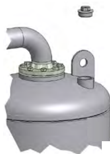
Removing plug from filler sleeve
